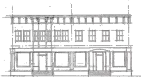
2-STORY FLAT ROOF BUILDING WITH BRACKETED PARAPET AND BAY WINDOW
